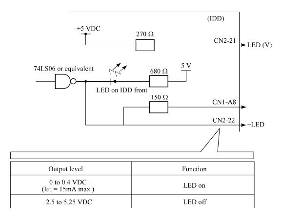
Figure 4.19 Output signal for external LED
